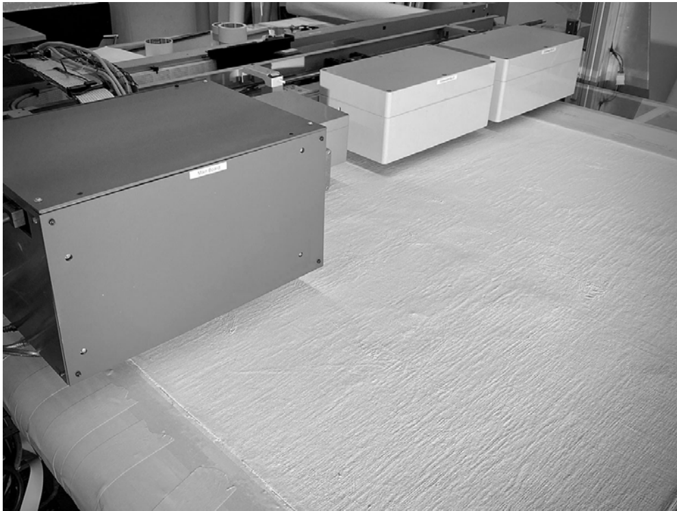
A flatbed inkjet printer begins to apply colour to a gesso texture - Photo: Nick Walkley
